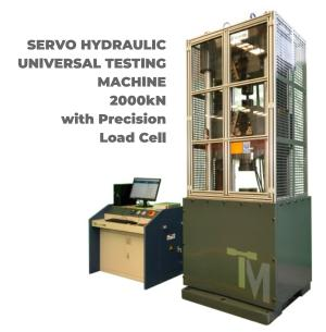
Machine offering high force capacity and precision for tensile, compression, and bending tests. With advanced hydraulic control and accurate load cells, this machine delivers reliable performance even for the most demanding industrial applications. It's designed for versatility and durability, ensuring consistent test results while handling large and complex samples with ease.
