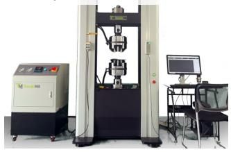
This system is designed for versatile material testing, offering precise control for tensile, compression, and flexural tests. With robust construction and advanced electronics, it ensures reliable performance across various sample types, making it suitable for both research labs and industrial applications. The user-friendly interface and flexible configuration options guarantee consistent accuracy and repeatability in diverse testing scenarios.
